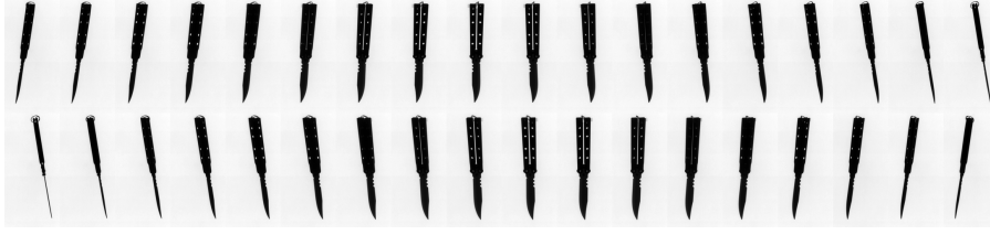
Fig. 8 A knife was rotated in 1^\circ and by each position an X-ray image was captured. In this figure, X-ray images at 0^\circ, 10^\circ, 20^\circ, \dots, 350^\circ are illustrated (see series B00008 of group Baggage).
